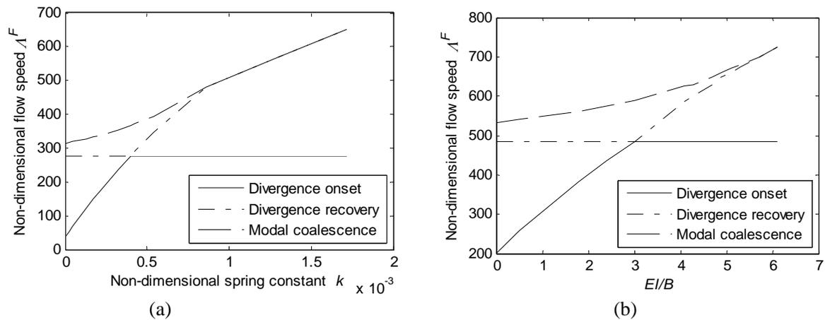
Figure 2: The variation of (non-dimensional) instability onset/recovery speeds with the magnitude of the added localised stiffening for (a) two-dimensional model (Fig. 1a) with an isolated spring, and (b) three-dimensional model (Fig. 1b) with a transverse stiffening strip.
