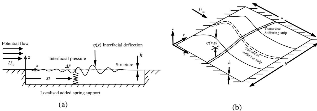
Figure 1: Schematics of the (a) two-dimensional (side view), (b) three-dimensional (isometric view) problems studied wherein a uniform flow interacts with a flexible panel that has localised stiffening; in (a) a spring support is added while in (b) a stiffening strip, that may be in either the transverse or streamwise direction, is bonded to the underside of the panel.
